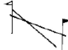
Top end of sloping pole higher than horizontal pole
