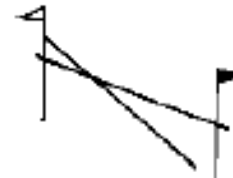
Top end of sloping pole higher than horizontal pole
